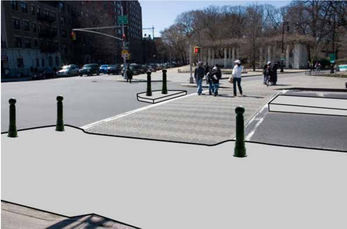
Figure 4. Drawing of Ocean Avenue at Parkside Avenue with curb extensions, raised median, pedestrian refuge, and bollards to calm traffic, shorten crossing distance and protect pedestrians
