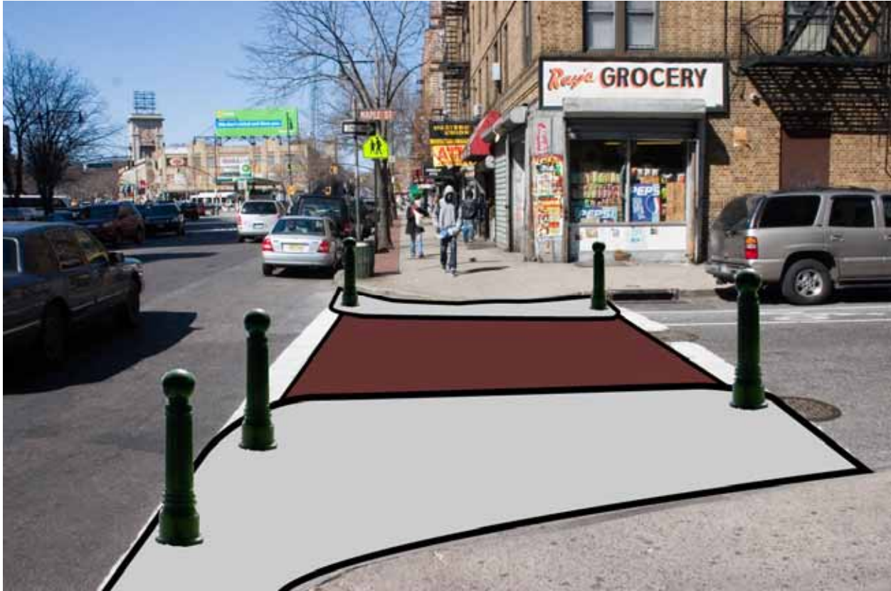
Figure 7. Drawing of Maple Avenue at Flatbush Avenue with curb extensions, raised median and bollards
