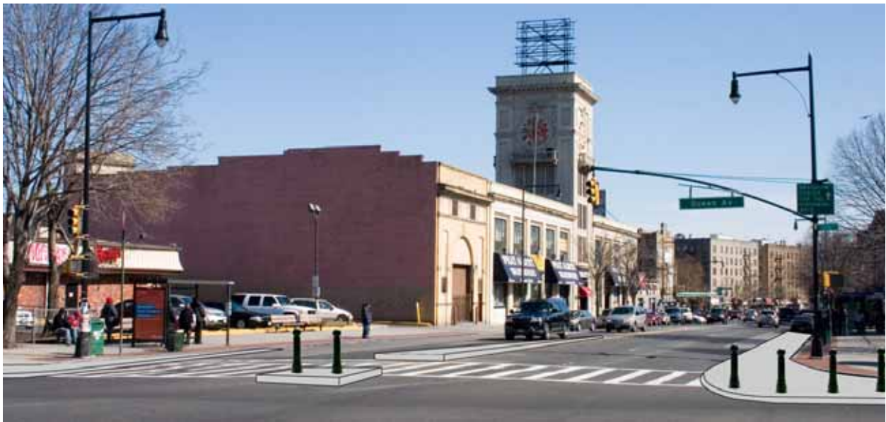
Figure 5. Drawing of Flatbush Ave. at Empire Ave. and Ocean Ave. with raised median, pedestrian refuge, bus bulb, and bollards
